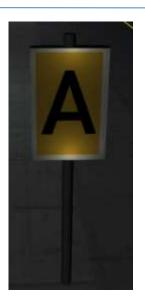
Lf 3 **"End disc":** end of the temporary slow speed section.
