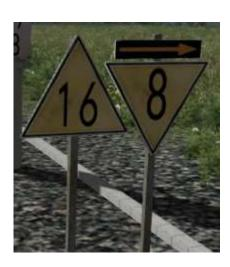
Lf 7 **"Speed table":** The speed indicated on the signal (number x 10) must not be exceeded after this signal.
