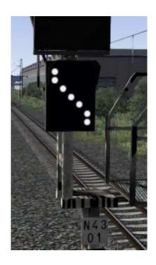
Zs 7 "Caution signal": Pass the disturbed or Hp 0 showing main signal without written command. Continue on sight.
